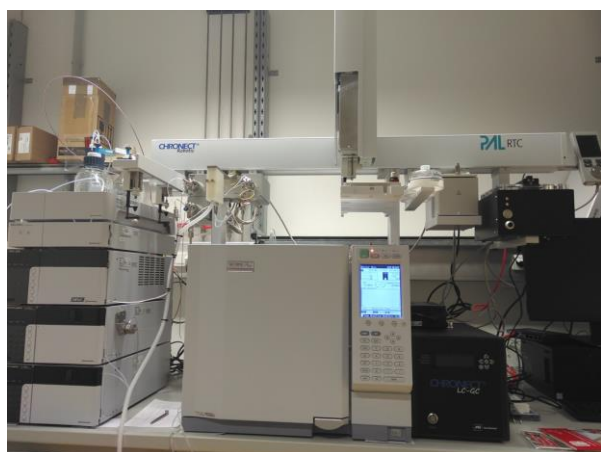
Fig. 3: LC-GC-FID System with automated epoxidation unit
