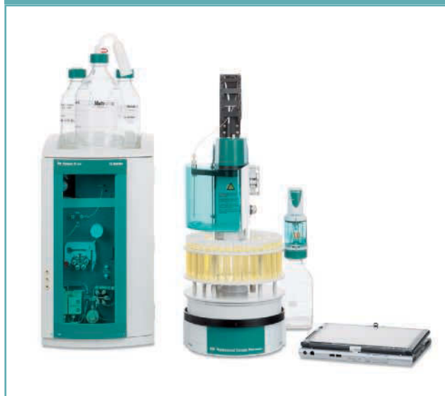
Figure 1: The 881 Compact IC pro with the 858 Professional IC Sample Processor with dialysis cell and 800 Dosino. Instrument control, data acquisition and processing were performed by MagIC Net software.
