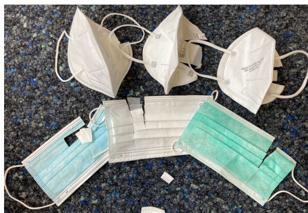
Figure 2: 6 different samples, from each style 3; these samples were examined for their content on polymers.
