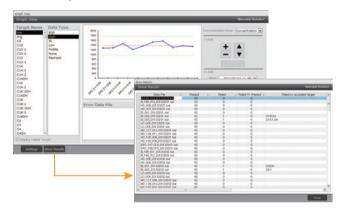
Accuracy is maintained using control samples. The permitted range is calculated from previously registered data; new data is then evaluated for adherence to the permitted range.
