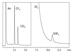
Fig. 4 Analysis of SF<sub>6</sub> Decomposition Gases (CF<sub>4</sub>: 310 ppm, SOF<sub>2</sub>: 107 ppm)
