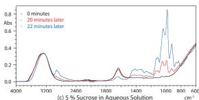
Fig. 5 Condensation Sampling Method – Time and Concentration Dependence of Sucrose ID
