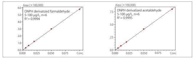
Fig. 3 Absolute Calibration Curves on Five Points
