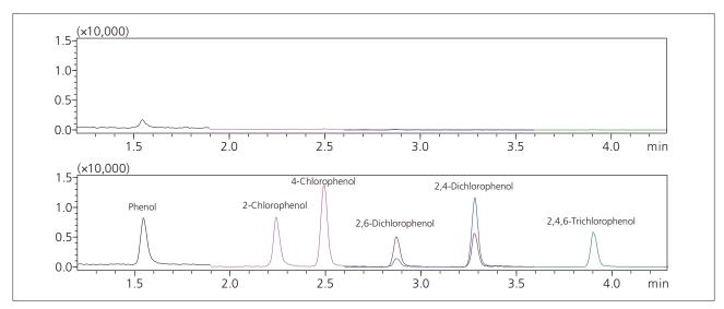
Fig. 3 Mass Chromatograms (MRM) of Drinking Water (Upper: Blank, Lower: 0.08 μg/L spiked)
