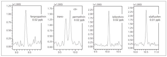
Fig. 2 MRM Chromatograms at Pyrethroid LOQs
