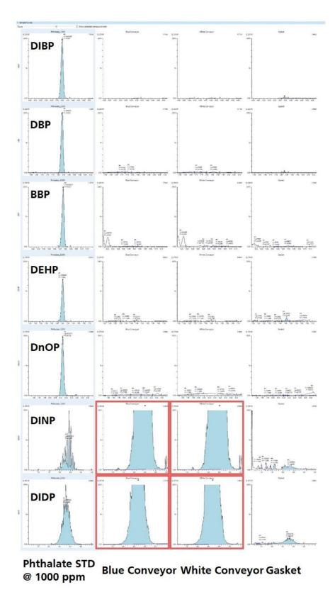
**Figure 5**: Quantitative analysis of the seven phthalate analytes in one standard and three polymer samples using the LabSolution Insight QAQC software. All the phthalate target compounds from three samples with unknown phthalate concentration are displayed with intensity scaled at the same level as phthalate standard at 1000 ppm. Phthalate content higher than 1500 ppm have been automatically flagged with a red box by the LabSolution Insight software.
