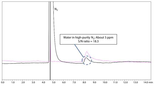
Fig. 4 Comparison of Chromatograms from High-Purity Nitrogen N<sub>2</sub> (Solid line) and Helium Standard Gas Containing Water at 10 ppm (Dotted line)
