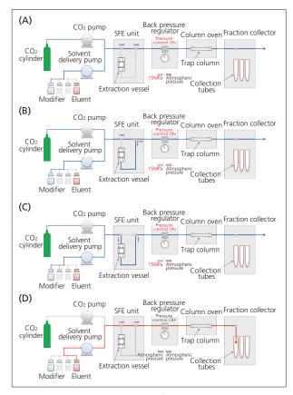
Fig. 1 Process Flow of SFE Extraction
