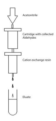
Fig. 3 Schematic Diagram of Elution Method Collection Method
