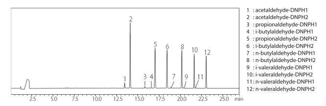
Fig. 4 Chromatogram for DNPH-Derivatized Lower Aliphatic Aldehydes (1 µg/mL Ethyl Acetate Solution)
