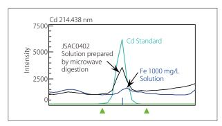
Fig. 1 Spectral Interference of Cd 214.438 nm
