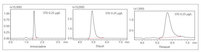
Fig. 2 MRM Chromatograms of Iminoctadine, Paraquat, and Diquat Standard Mixture
