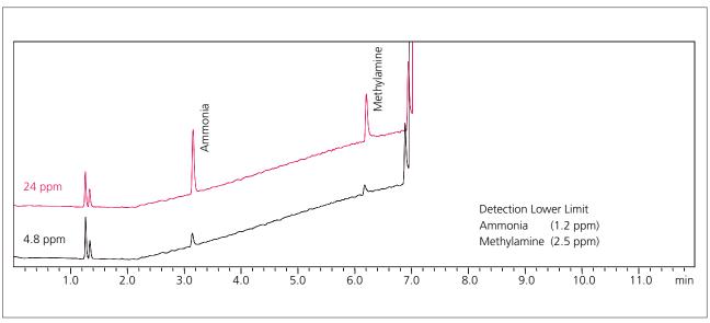
Fig. 1 Chromatograms of 4.8 ppm and 24 ppm Standard Solutions
