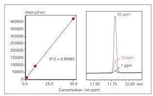
Fig. 9 Linearity of Formic Acid in Methanol (1, 10, 50 ppm)
