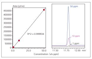
Fig. 6 Linearity of Formic Acid in Acetone (1, 10, 50 ppm)
