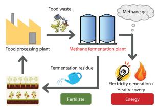
Fig. 1 Schematic of Recycling System Utilizing Methane Fermentation
