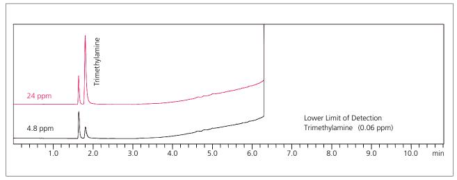
Fig. 3 Chromatograms of 4.8 ppm and 24 ppm Standard Solutions
