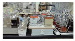
Fig. 5 Laboratory-scale Methane Fermentation Test System
