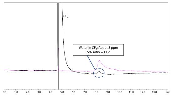
Fig. 3 Comparison of Chromatograms from CF<sub>4</sub> Chlorofluorocarbon Gas (Solid line) and Helium Standard Gas Containing Water at 10 ppm (Dotted line)
