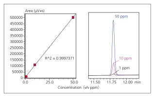
Fig. 8 Linearity of Formic Acid in Acetonitrile (1, 10, 50 ppm)
