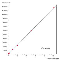
Fig. 3 Linearity of SF<sub>6</sub> in the Atmosphere (0.1 to 50 ppm)
