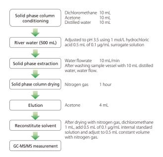
Fig. 3 River Water Sample Pretreatment Flow
