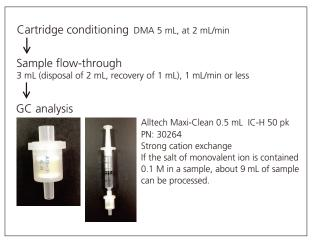
Fig. 2 Pretreatment Procedure Using Cation-Exchange Cartridge
