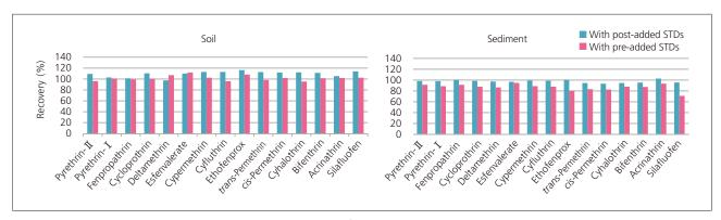
Fig. 4 Recoveries from Soil and Sediment
