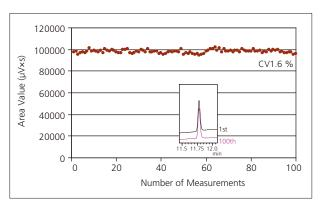
Fig. 5 Repeatability of Peak Area with 10-ppm Formic Acid / Acetone Solution at the Hundredth Analysis
