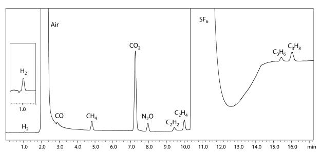
Fig. 1 Analysis of Impurities in SF<sub>6</sub>
