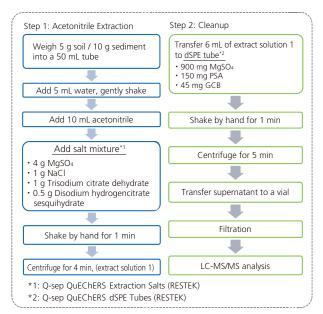
Fig. 3 Sample Preparation Using QuEChERS Method
