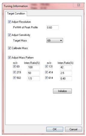
**Figure 3B**: Recommended BFB Tune Conditions Using *m/z* 69 as the Target Mass and Mass Pattern Adjustment
