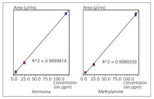
Fig. 2 Linearity of Ammonia and Methylamine (4.8, 24, 120 ppm)
