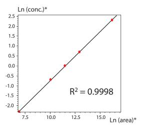
\* In the analysis of sulfur compounds using an FPD detector, the output is proportional to the square of the sulfur concentration. Thus the natural logarithm for both concentration and area should be plotted.
