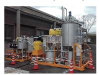
Fig. 2 Transportable Methane Fermentation Pilot Plant
