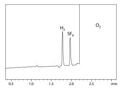
Fig. 2 Analysis of Trace SF<sub>6</sub> (0.1 ppm) in the Atmosphere
