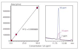
Fig. 7 Linearity of Formic Acid in N,N-Dimethylacetamide (1, 10, 50 ppm)
