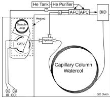
Fig. 1 Trace Moisture Analysis System
