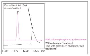
Fig. 4 Comparison of Formic Acid Peak Shapes Before and After Column Phosphoric Acid Treatment
