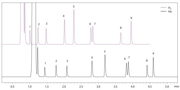
Fig. 3 Chromatograms of Mixed Solution of Organic Solvents (Pink: H₂ Carrier Gas, Black: He Carrier Gas)
