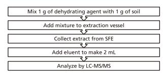
Fig. 3 Process Flow from Pretreatment to Analysis
